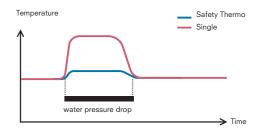
By comparison with the SINGLE product, SAFETY THERMO produces a smaller range of temperature fluctuations during bathing, even when the water pressure drops due to a toilet flushing.
